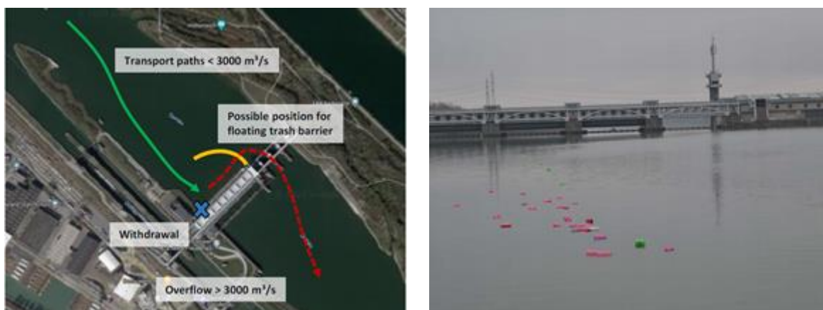
Figure 7 - Sketch describing a possible positioning of a floating macro plastic barrier at the HPP (left); Tracer study with GPS-tagged floating items (right) in front of the HPP Freudenau, Vienna (right)
