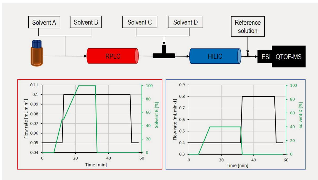
Figure 1: Schematic presentation of the instrumental setup with flow rates and gradients of RPLC (bottom left) and HILIC (bottom right).
