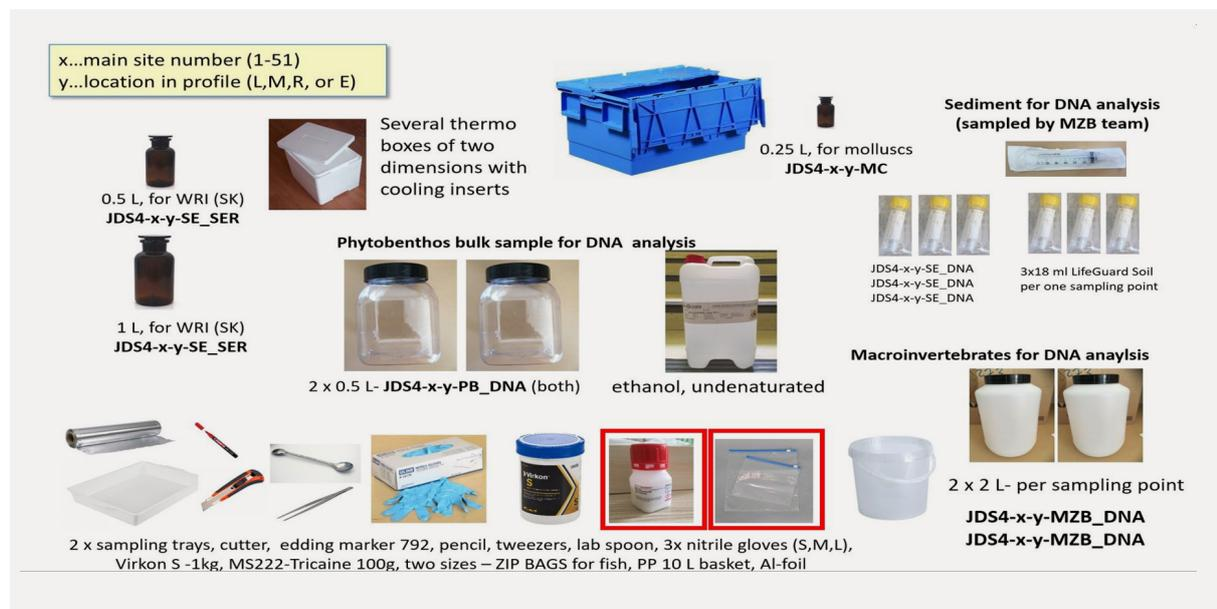
Figure 1: An example of infographic explaining the content of the box with sampling vessels, chemicals and materials distributed to the National Teams prior to the survey.
