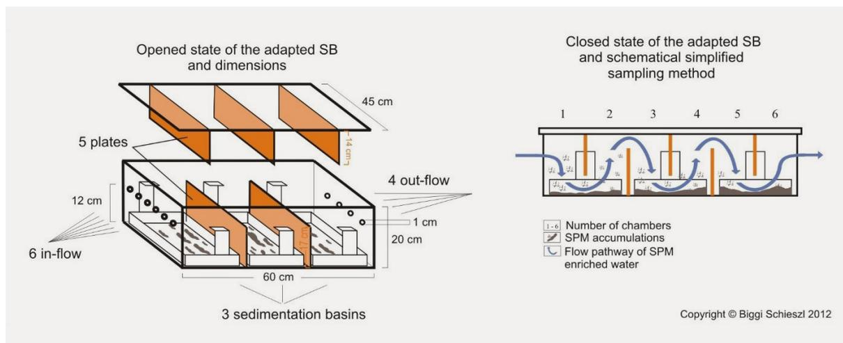
Figure 1: Basic scheme of the sedimentation box used for collection of SPM samples for the German Environmental Specimen Bank (ESB) (Schubert et al. 2012).
