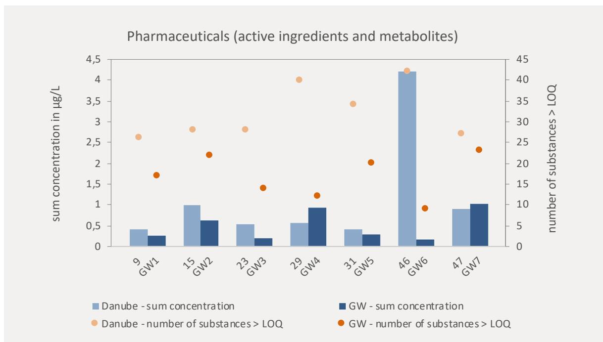
Figure 4: Sum concentration (in µg/L) and number of substances > LOQ for the corresponding monitoring sites Danube/groundwater.
