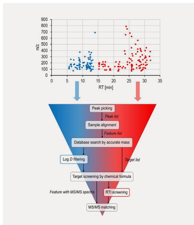
Figure 2: Data processing workflow from nontargeted raw data to a list of polar as well as nonpolar candidates present in the JDS4-7 sample.
