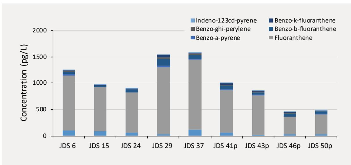
Figure 6: Longitudinal profile of  $C_{free}$  concentrations priority PAHs along the Danube.
