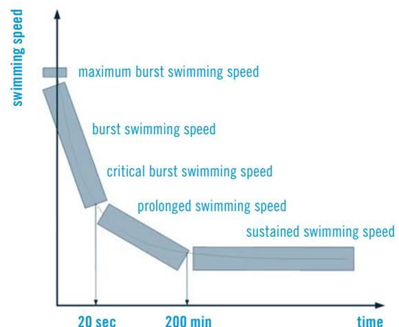
The (critical) burst swimming speed of the “weakest swimmer” among the river-specific fish-fauna should be used to define the thresholds of flow velocities within the migration corridor of the FP. The “weakest” are usually juveniles and small fish species (e.g. bullhead and stone loach) (BMLFUW 2012).
