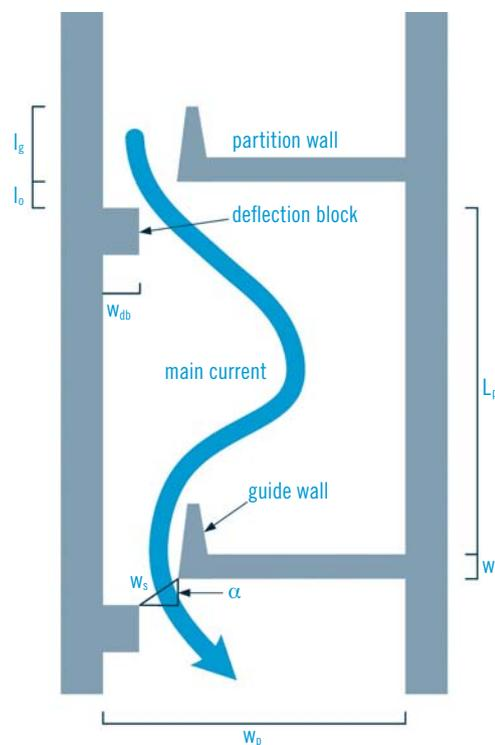
The maximum acceptable energy dissipation of the respective river type has to be considered. The slots usually include a hydraulic steering device to ensure an oscillating main current using the entire pool volume for a low-turbulence energy transformation (Heimerl and Hagemeyer 2005, Heimerl et al. 2008) as shown in Figure 12:
