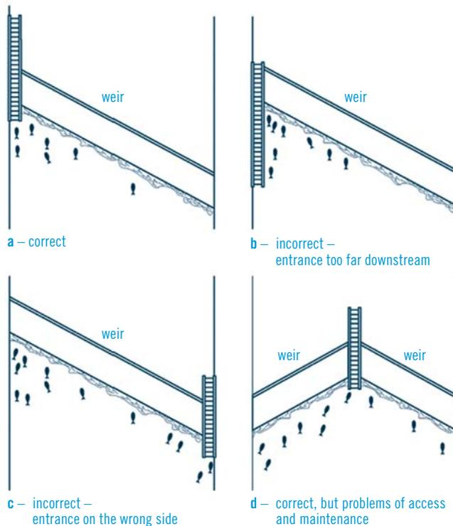
There is at least one optimal position (key position) of the entry that lies in the interface between the downstream limits of the barrier (or the turbulent zone) and the longitudinal corridor of migration (Dumont et al. 2005). Furthermore, directly at the FP entry, the attraction flow should be as parallel as possible to the main current ( $< 30^\circ$ ) (DWA 2010, draft).
