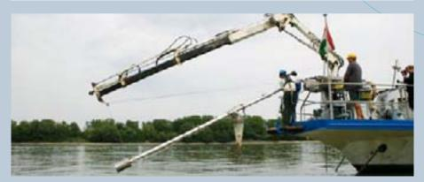
The 'air-lift' sediment sampler, the Argus's most prominent feature, was used for the first time for Danube sampling. *Credit: ICPDR*
