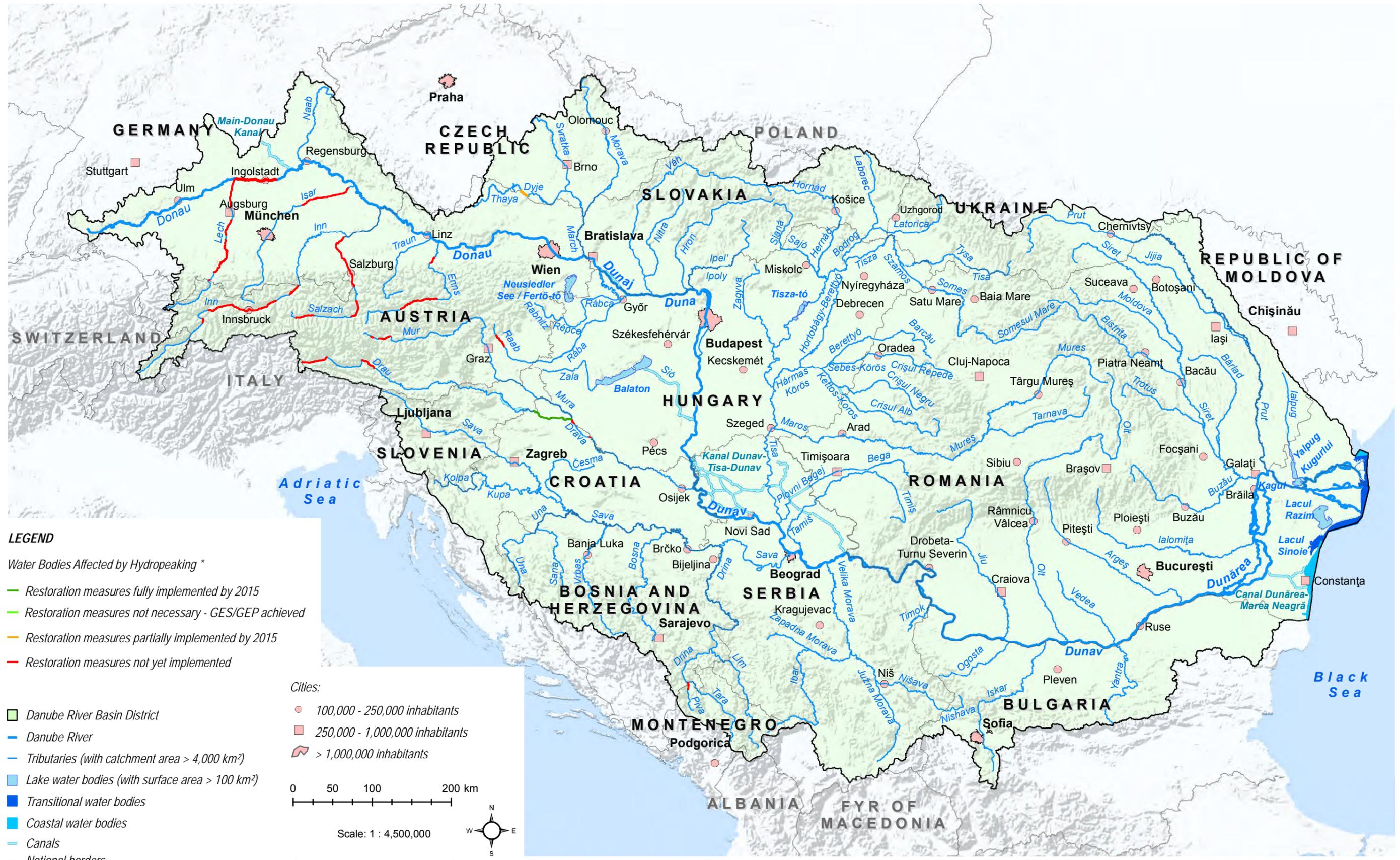
\* Significant hydrological alterations with water level fluctuation >1m/day or known/observed negative effects on biology. This map illustrates full water bodies which are affected by hydropeaking. The exact locations of individual pressures from hydropeaking are not visualised.
