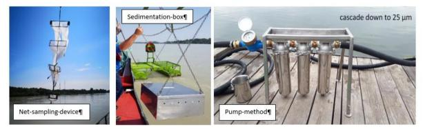
Figure 1 – Devices of the 3 sampling methods applied and compared within the Tid(y)Up project
