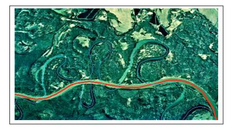
Figure 1 Example of channel straightening - modification of Morava river, - new river course (indicated in red), - original river course (indicated in blue)
