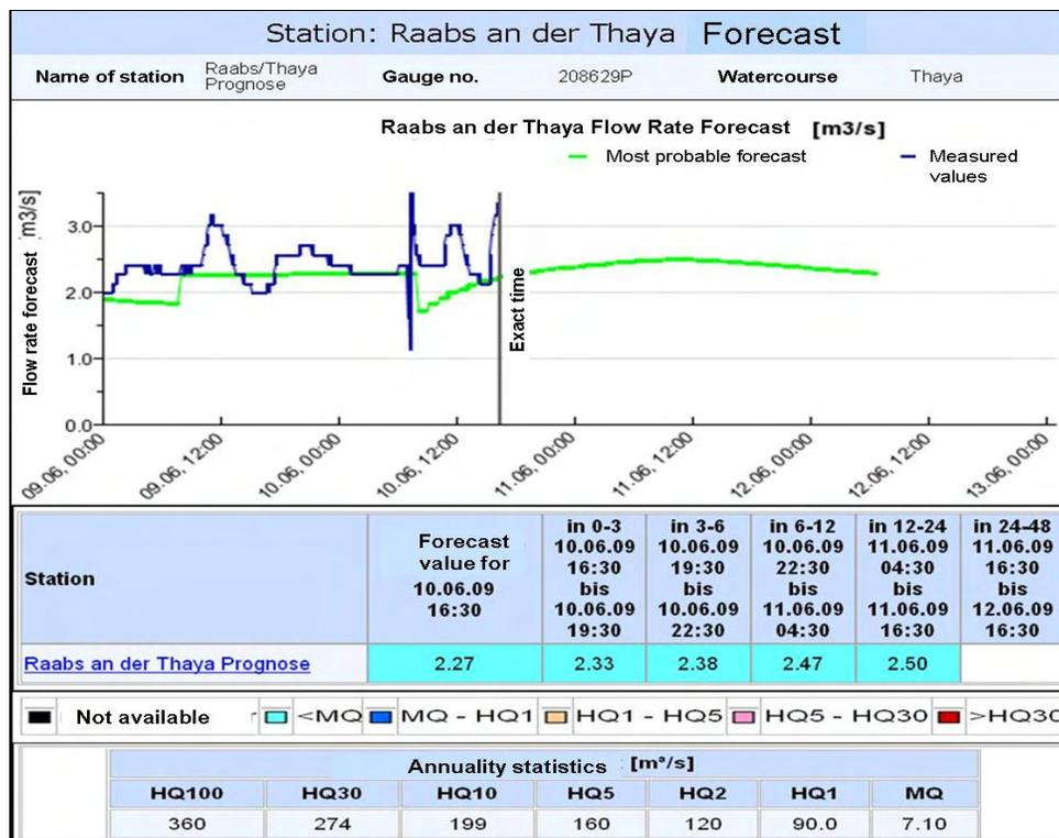
Fig. 3-7: Example of an online flood forecast of the Hydrographic Service of Lower Austria (Source: Homepage of the Hydrographic Service of Lower Austria, modified: Revital ZT)
