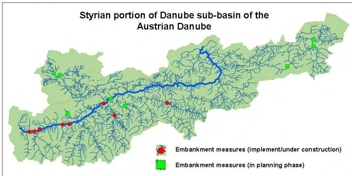
Fig. 3-4: Embankment measures in the Styrian portion of the Danube sub-basin
