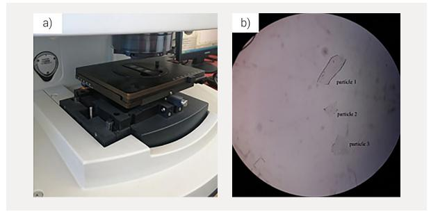
Figure 3: MicroATR spectroscopy (a) and particles prepared for analyses (b).
