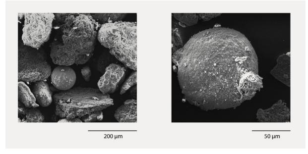
Figure 4: Scanning electron micrographs of Kostolac fly ash at 500x and 1500x magnification exhibiting both irregularly shaped particles with vesicular texture and smooth spherical particles of different sizes.
