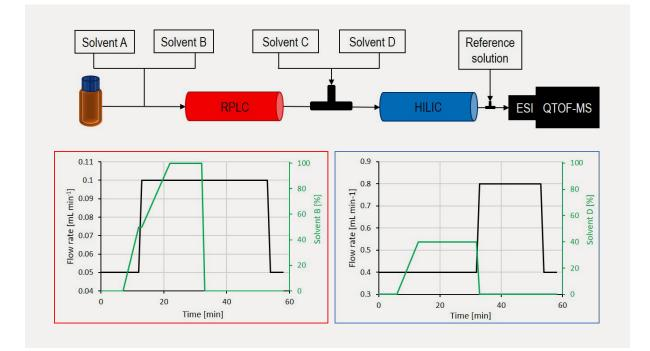
Figure 1: Schematic presentation of the instrumental setup with flow rates and gradients of RPLC (bottom left) and HILIC (bottom right).
