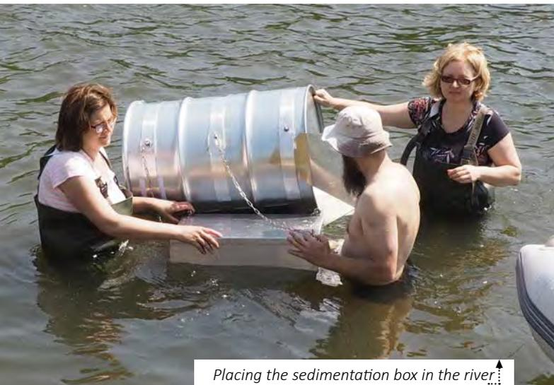
Placing the sedimentation box in the river<sup>2</sup>
