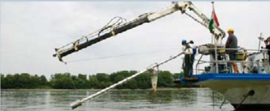
The 'air-lift' sediment sampler, the Argus's most prominent feature, was used for the first time for Danube sampling. *Credit: ICPDR*
