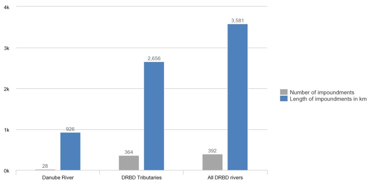
For the Danube River, impoundments are the key hydrological pressure type causing significant alterations. 926 km of its entire length (of 2,857 km) are impounded (representing 32% of the length) by 28 barriers. In fact, impoundments are the major hydrological pressure type for the Danube River.
