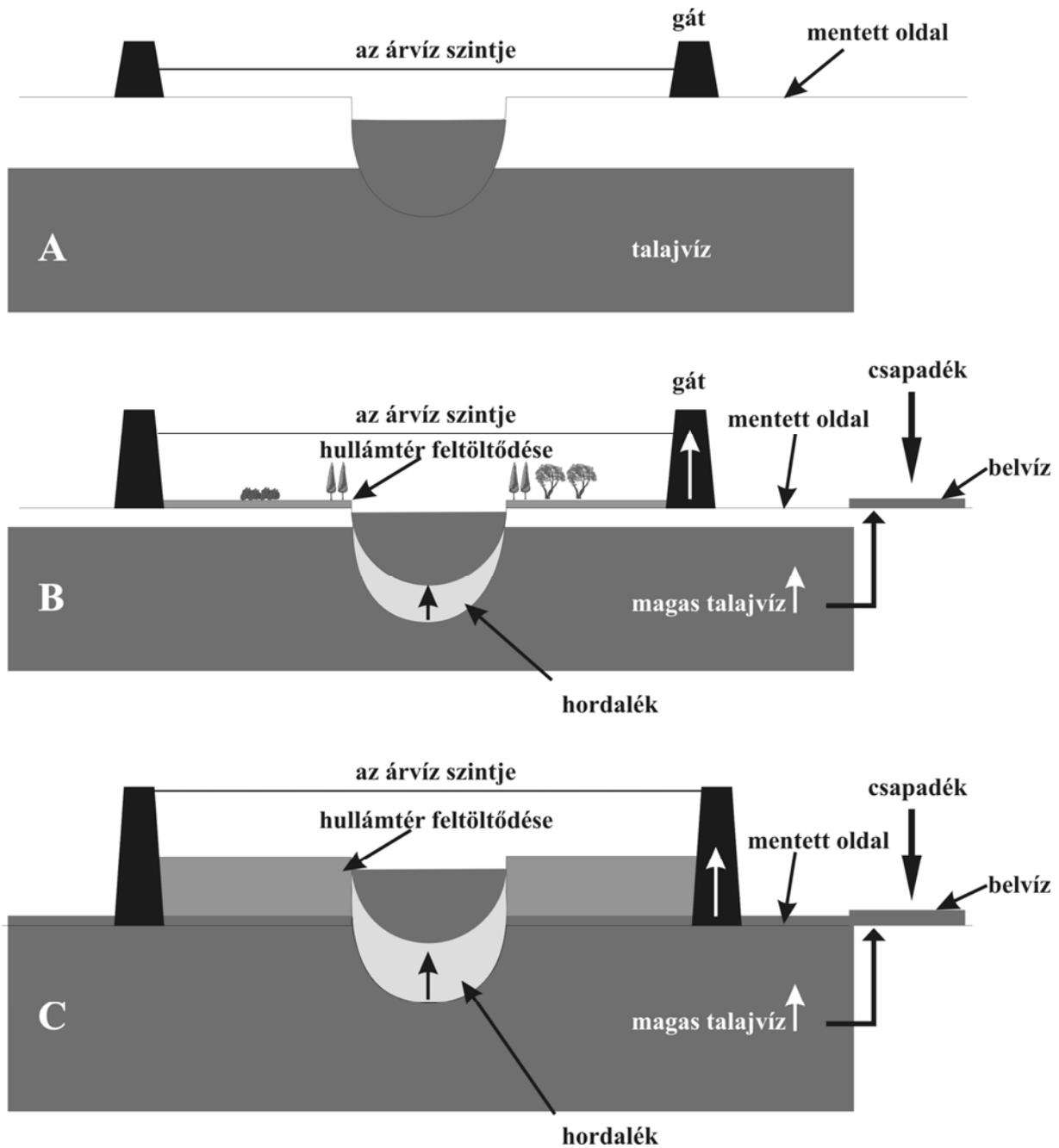
**Figure 12: System feedback of river regulations**
