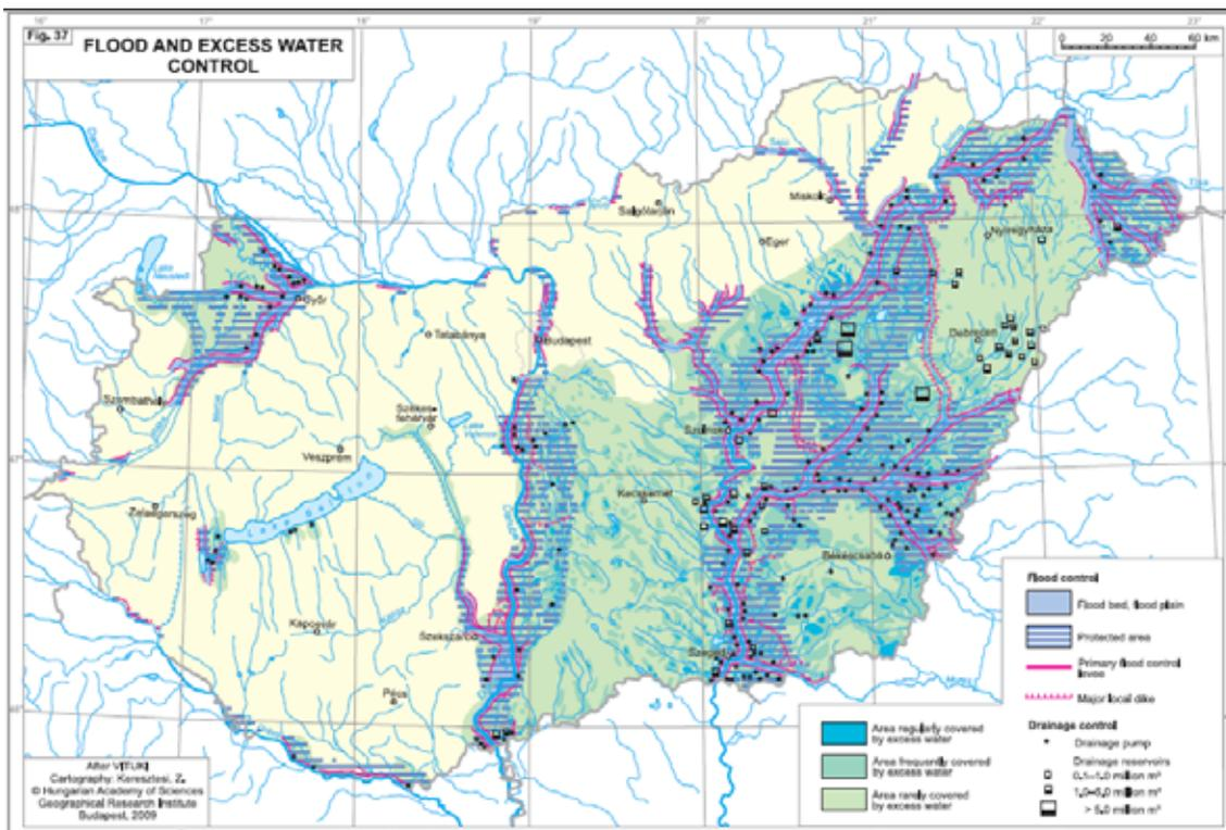
**Figure 10: Areas protected by flood control works and exposed to excess water in Hungary (Alföldi 2009: p 54)**
