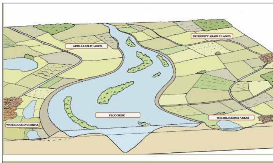
Figure 25: High stage river bed of a trained river
