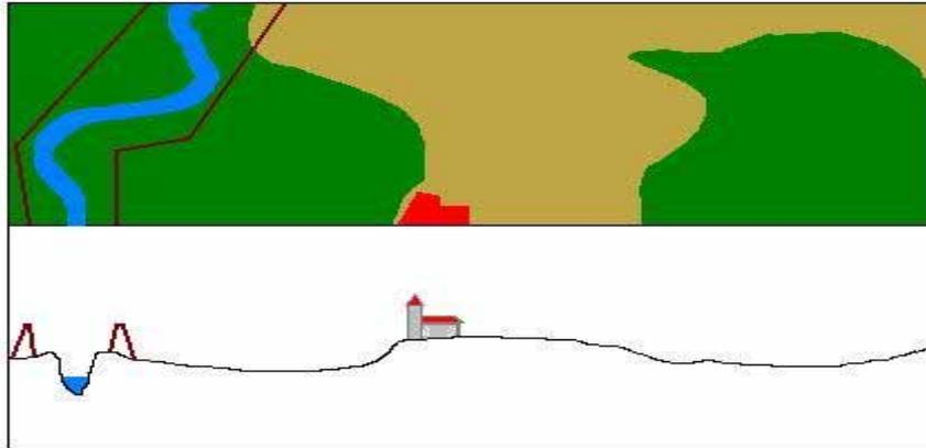
**Figure 28: Trained river on the flood plains at low water stage**
