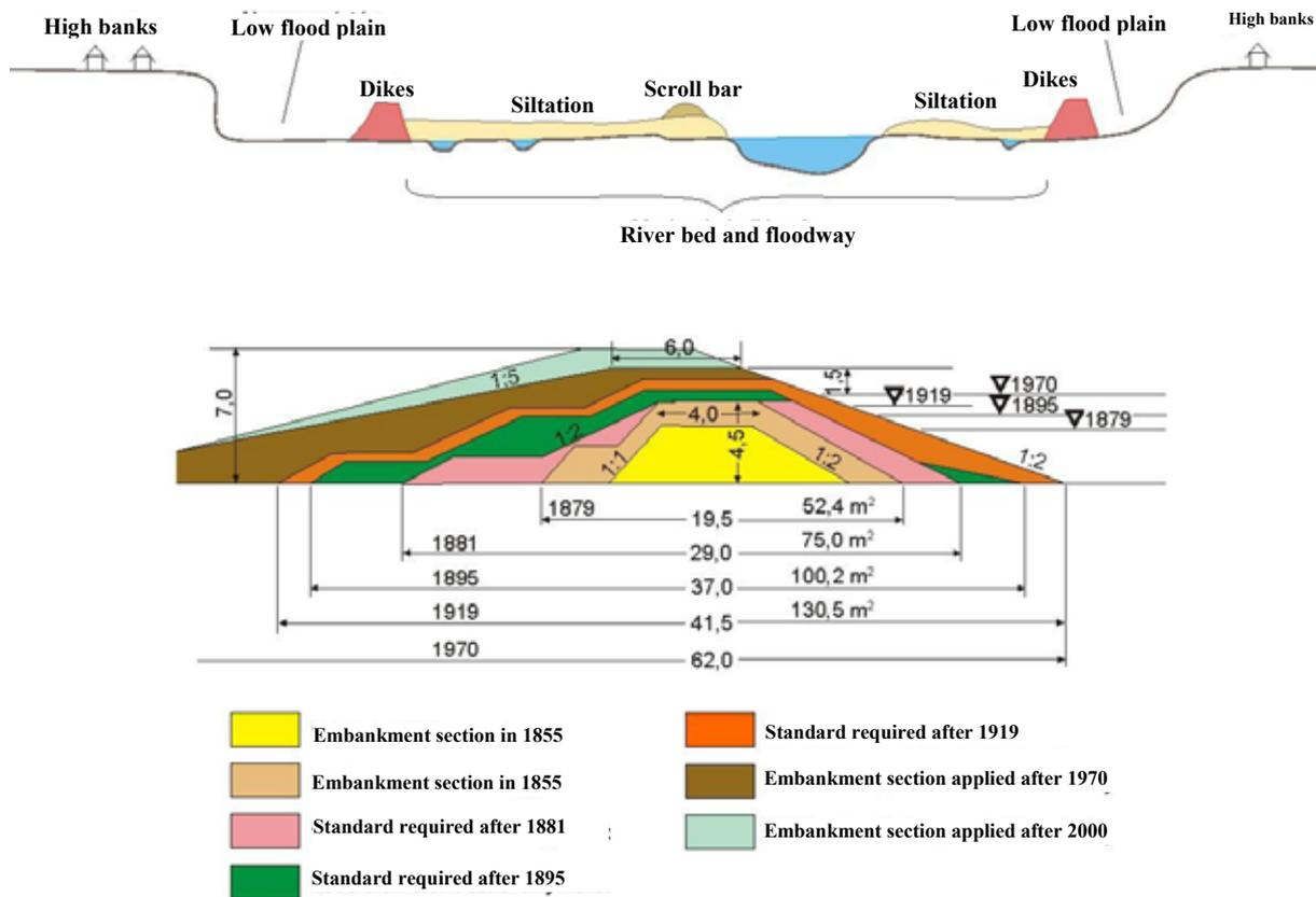
Figure 7: Increasing the height of flood control levees, adapted from Vágás, I and Schweitzer (2002)
