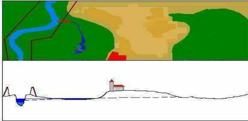
**Figure 31: The theoretical concept of ILD: controlled discharge of water starts at mean water level from the mean-stage river bed**
