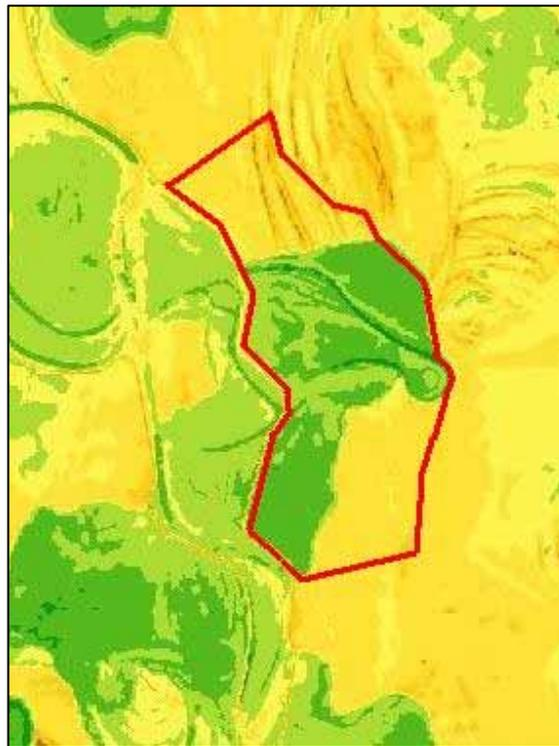
**Figure 50: The ground area of the Tiszaroff reservoir on a contour map. Green is deep floodplain, yellow is higher banks**
