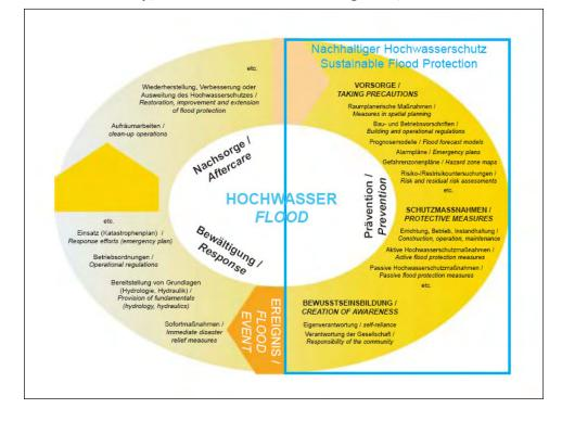
Fig. 3-1: Sustainable flood protection (Diagram: Federal Ministry of Agriculture, Forestry, Environment and Water Management, 2006b)
