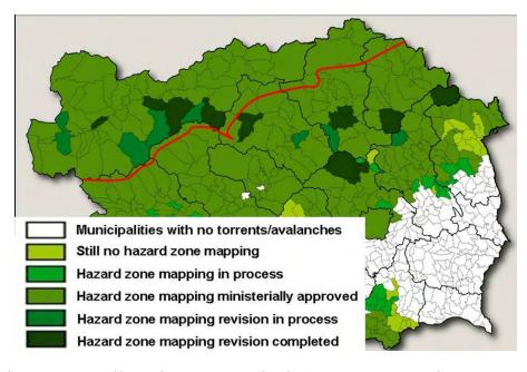
Fig 3-1: Current status of hazard zone mapping by the Forest Engineering Service in Torrent and Avalanche Control in Styria (Image: Styrian Section of Torrent and Avalanche Control)
