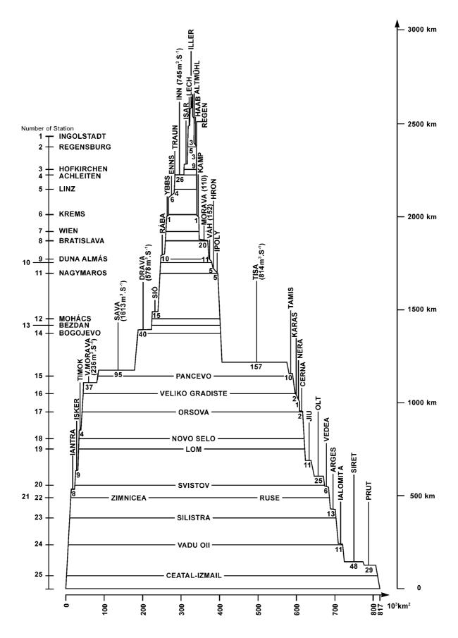
Figure 1.1-2Diagram of Area, Sequence and Length of Danube Tributary BasinsSource: Redrawn from Stancik Andrej and Slavoljub Jvanovic at al. 1988, Hydrology of the Danube River
