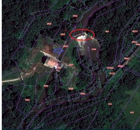
Figure 4: The mill by Straža. Red circle: the barrage, blue arrow: diversion channel
