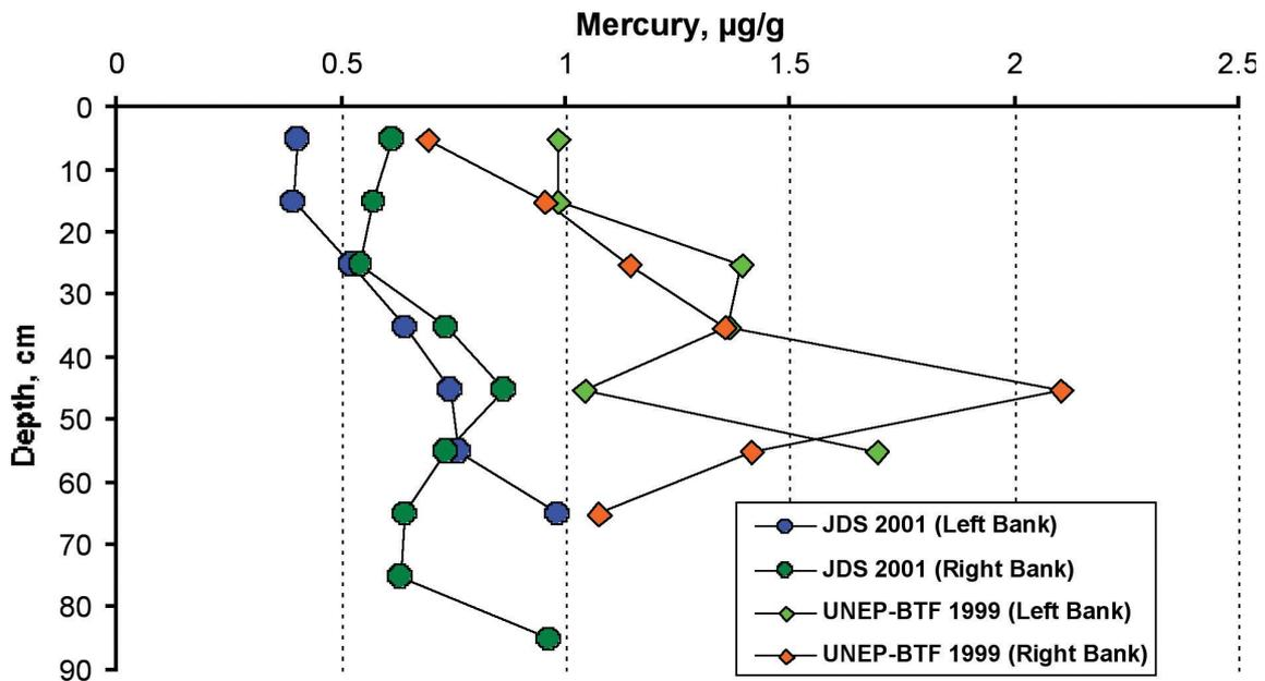
FIGURE C2.3.-16: Comparison of mercury concentrations determined in 10 cm layers of sediment cores sampled on the left and the right banks of river km 1077 (Iron Gate Reservoir)
