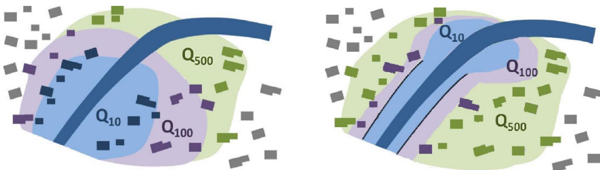
Figure SI4: Example of buildings in flooded areas at discharges of return period 10, 100 and 500 before and after the implementation of measure (flood protection dams: depicted by black lines)
